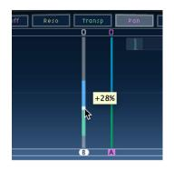
To adjust the stereo balance in stereo input/stereo output configurations: Drag the Pan parameter—which appears as a dot on the tap—up or down the tap to adjust the stereo balance.
