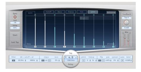
You can move a tap backward or forward in time or completely remove it.
