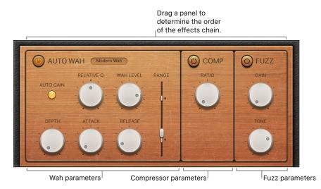
Fuzz-Wah effects work in series—where the output of one effect is fed into the next in an effects chain. The routing order lets you choose whether a distorted signal should be wah-filtered (for funkier sounds) or the wah-filtered sound should be distorted (for screaming sounds), for example.
