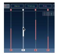
When the highpass filter cutoff frequency value is lower than that of the lowpass cutoff frequency, only one line is shown. This line represents the frequency band that passes through the filters—in other words, the filters act as a bandpass filter. In this configuration, the two filters operate in series which means the tap passes through one filter first, then the other.
