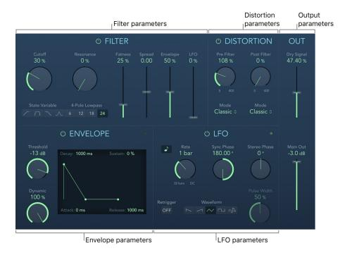
The AutoFilter window is divided into Filter, Envelope, Distortion, LFO, and Output parameter sections.
