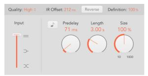
In Logic Pro, rotate the Length knob to set the length of the impulse response—sampled or synthesized.
